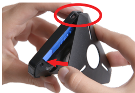
Replace the lid, starting with the hook
